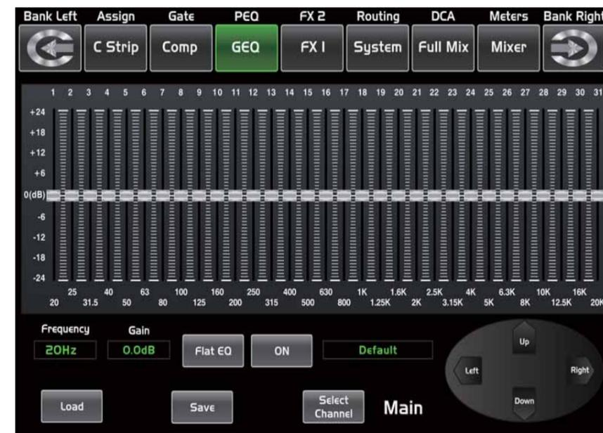
The digital mixer features MAIN Stereo, AUX Mono, 31-band, 1/3 octave graphic EQs. The 31 bands range from 20Hz to 20 KHz. There is 1 MAIN Stereo GEQ, 8 AUX Mono GEQs in 24-bit/48 kHz sample rate.
