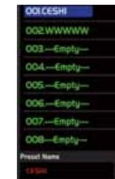
This items show names of preset, when you select a preset, its name will show on the bottom box, then touch Load control on the screen to load the selected preset to corresponding controls.
