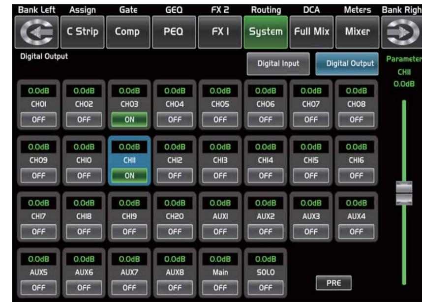
When you select a channel as digital output, OFF will switch to ON, the background of ON will illuminate. The screen will give clues if no digital card inserted in, and the Digital Out function can not enable either.
