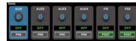
Touch AUX1-4 and FX1-2 on the LCD screen or press corresponding button on the panel to assign input channel audio to these channels or buses. To adjust output level of the channel audio, you can rotate Parameter Adjust knob on the panel.
