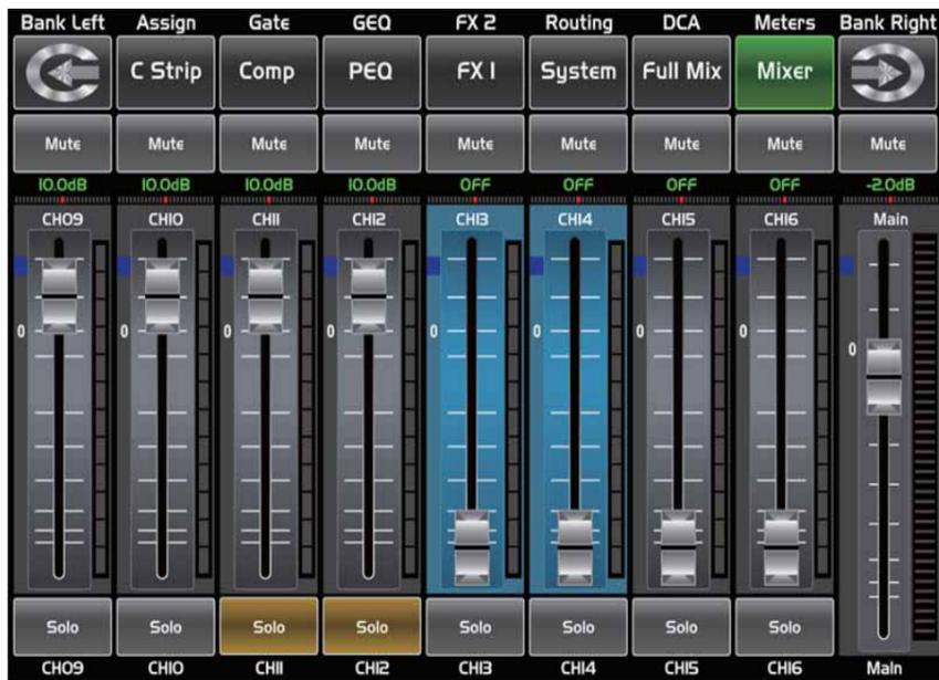
Touch this icon to switch channels and enter corresponding Long Faders page, in which you can adjust channels' basic function like pan, solo, mute, level and rename the channel, etc.
