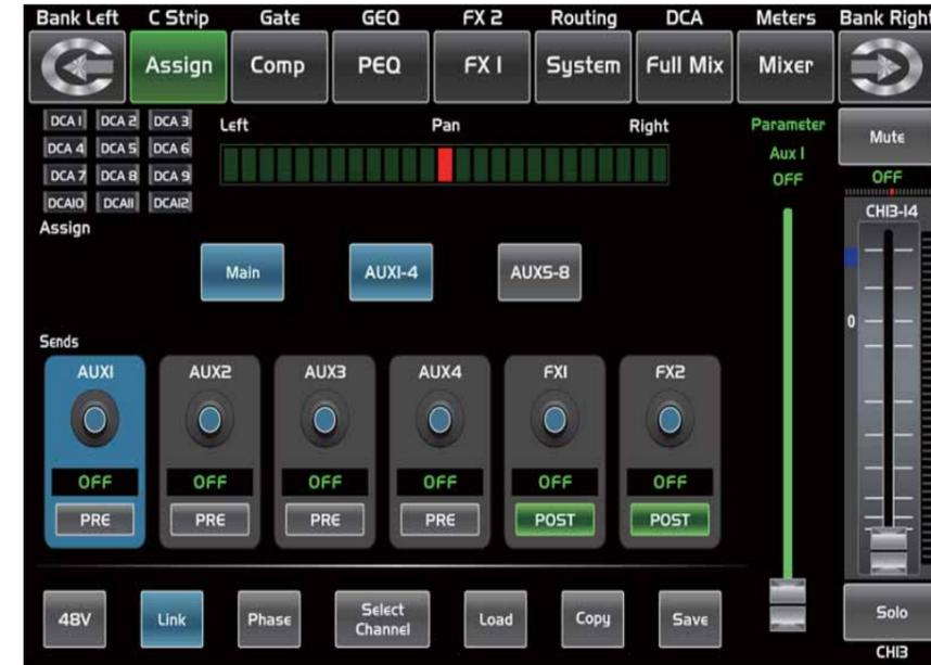
Touch Main, AUX1-4 or AUX5-8 on the LCD screen or corresponding button on the panel to assign input channel audio to these channels or buses. They will illuminate synchronizing with buttons in Assign area on the panel after pressed. To adjust output level of the channel audio, you can rotate Parameter Adjust knob or corresponding Main, AUX1-4 or AUX5-8 knobs on the panel.
